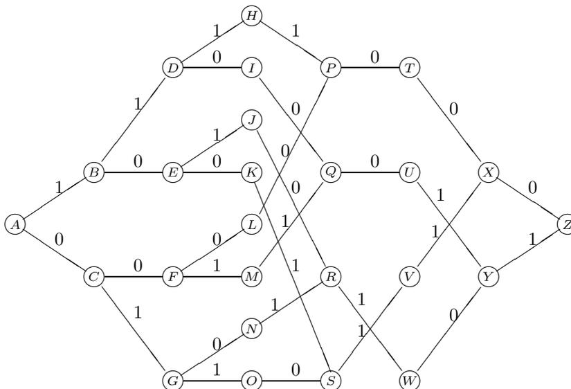
Figure 1: A trellis for the dual Hamming code
