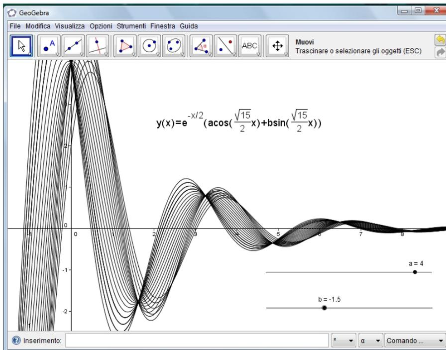
FIGURA 3.  $y_0(x) = e^{-x/2} \left( c_1 \cos \left( \frac{\sqrt{15}}{2} x \right) + c_2 \sin \left( \frac{\sqrt{15}}{2} x \right) \right)$
