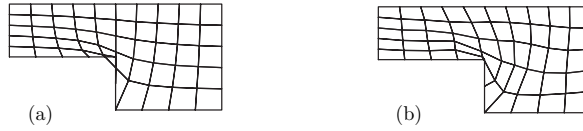
Fig. 5: The grid generated for region Backstep with N = 5 and M = 10 : (a) grid obtained with parameters p_L = p_A = p_O = 2 , (b) grid obtained with parameters p_L = 8, p_A = p_O = 2 . In both cases we have folded grids but in (a) the folding is more severe than in (b).
