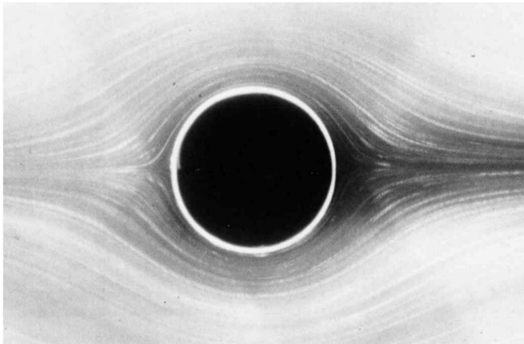
Shear flow past an obstacle at  $Re = 0.16$
