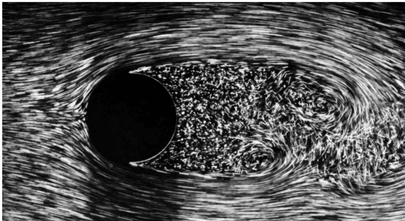
Turbulence past an obstacle at  $Re=2000$
