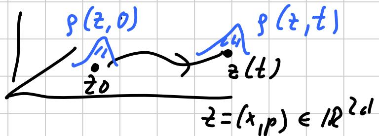
$\rho(z, t)$  = push-forward of  $\rho(z, 0)$  under flow  $\Phi(z, t) = \text{soln to (Ham.)}$
