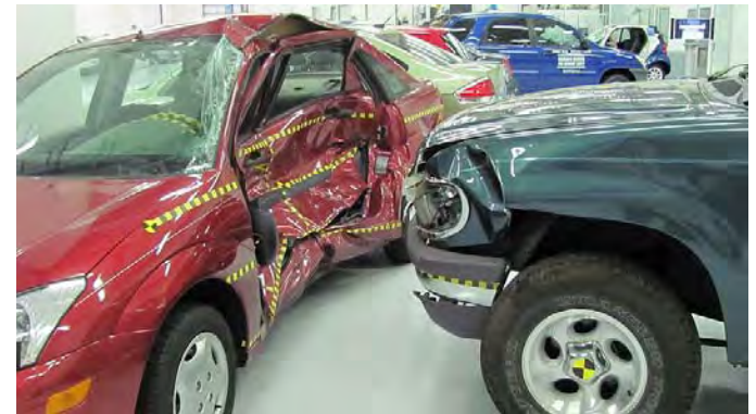
Side-impact test of 1996 Ford Explorer vs. 2000 Ford Focus
