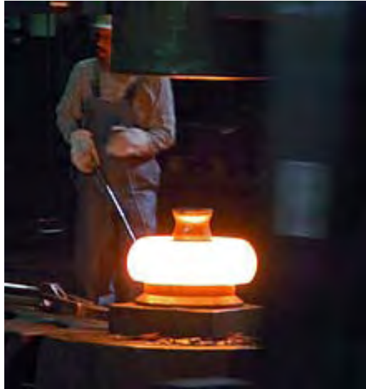
Metal ingot after forging
