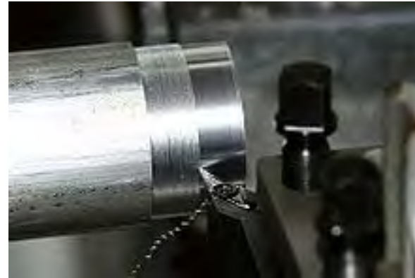
Lathe cutting metal from workpiece
