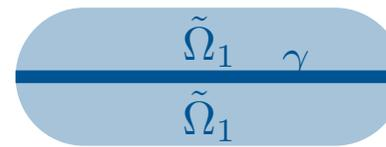
$$\begin{aligned} L_1 u_1 &= f_1 && \text{in } \tilde{\Omega}_1 \\ L_\gamma u_\gamma &= f_\gamma && \text{on } \gamma \\ &&& + \text{coupling conditions on } \gamma \end{aligned}$$
