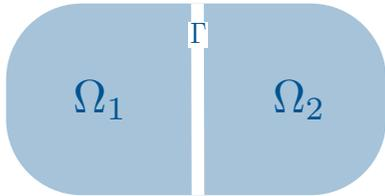
$$\begin{aligned} Lu_1 &= f_1 && \text{in } \Omega_1 \\ Lu_2 &= f_2 && \text{in } \Omega_2 \\ &&& + \text{coupling conditions on } \Gamma \end{aligned}$$
