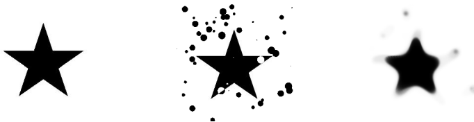
Figure: Original star shape (top), star shape with random droplets (center) and filtered by APMCM (bottom)
