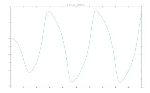
Here is the Euler discretion of the Van der Pol Oscillator with time step 0.1 second,
