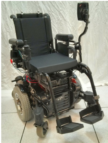
Shared control smart wheelchair for older adults with cognitive impairments [Viswanathan et al, Autonomous Robots 2016].
