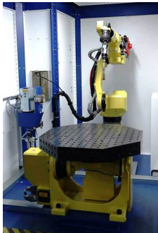
Printing robot and work pieces, by courtesy of Johannes Buhl, BTU Cottbus-Senftenberg
