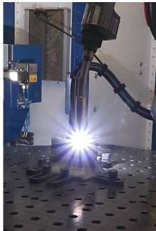
Printing robot and work pieces, by courtesy of Johannes Buhl, BTU Cottbus-Senftenberg
